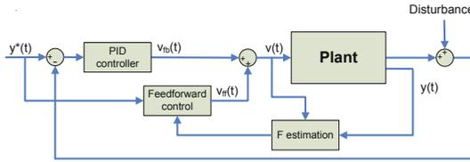
**Fig. 6.** i-PID control scheme
