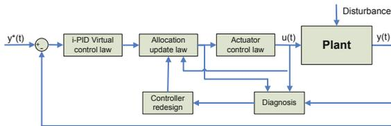
Fig. 7. Fault tolerant control for an effort allocation based control scheme
