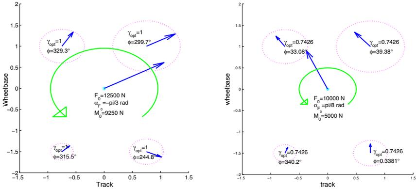
Fig. 3. Examples of efforts allocation with the same load distribution, but with different targets
