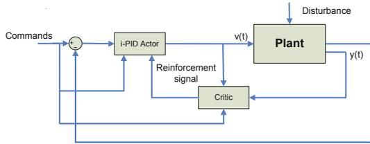
Fig. 5. Reinforcement learning scheme for Global Chassis Control
