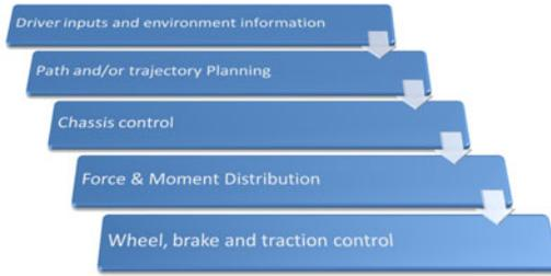
**Fig. 2.** Flowchart of the proposed control architecture
