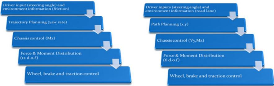
Fig. 4. Flowchart for an ESP in a 4WS vehicle (left) and a Lane Keeping in an AFS car (right)
