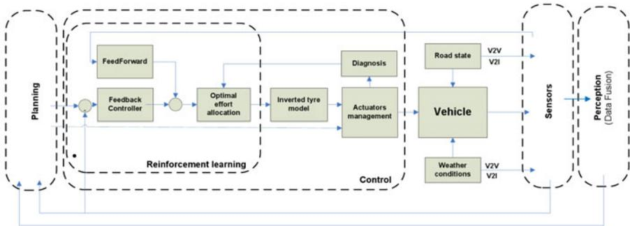
Fig. 1. Modular control architecture for automated vehicles
