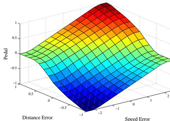
Fig. 4. Speed control surface.
