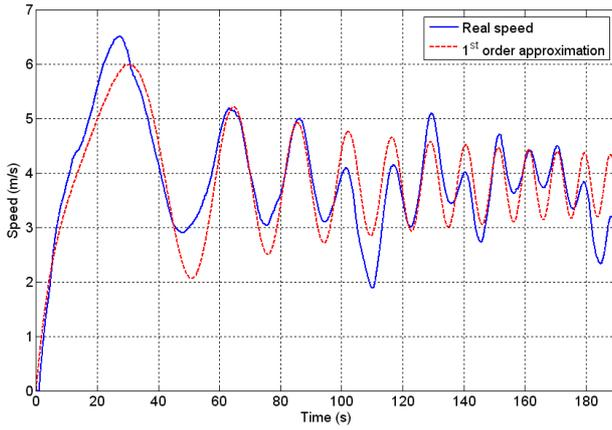
Fig. 3. Experimental vehicle response for the identification of its longitudinal dynamics
