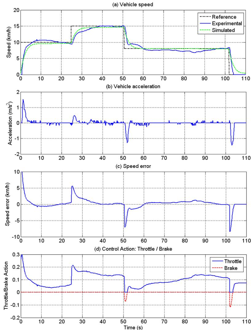
Fig. 9. Vehicle response by applying the  $PI^\alpha$  controller: (a) Speed –experimental and simulated– (b) Acceleration (c) Speed error (d) Control action
