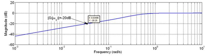
Fig. 5. Magnitude of the sensitivity function  $S(s)$
