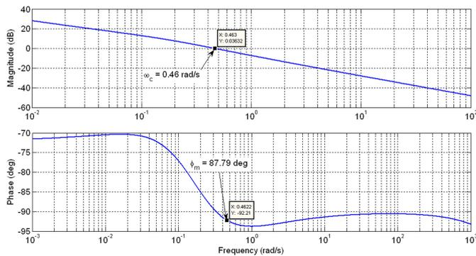
Fig. 4. Bode plot of the controlled vehicle by applying the designed  $PI^\alpha$  controller
