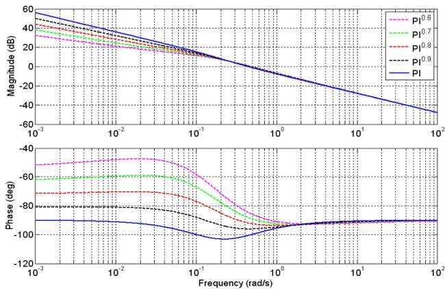
Fig. 7. Bode plots by applying a  $PI^\alpha$  controller with different values of the order  $\alpha$
