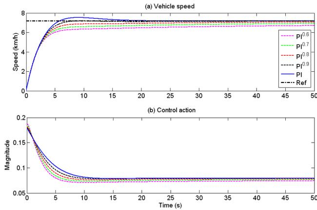
Fig. 6. Step responses by applying a  $PI^\alpha$  controller with different values of the order  $\alpha$ : (a) Vehicle speed (b) Control action
