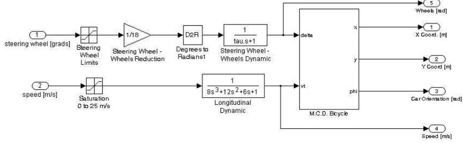
**Fig. 2.** Expanded view of the car model.
