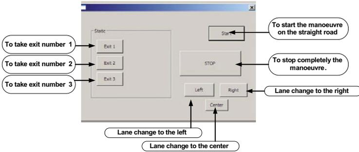
Fig. 2. Interactive interface of the roundabout maneuvers
