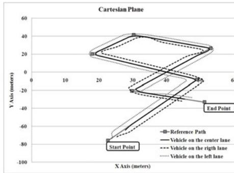
**Fig. 4.** Lane keeping in the central, right and left line
