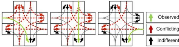
**Fig. 2.** Conflicting lights for a light to turn green for a left-turn (left), straight (centre), and right-turn (right) manoeuvre. A light cannot be turned green while any of its conflicting lights is green or amber.
