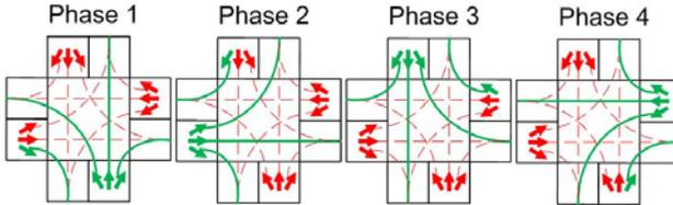
Fig. 3. Four phases used in Fixed Time Prioritization
