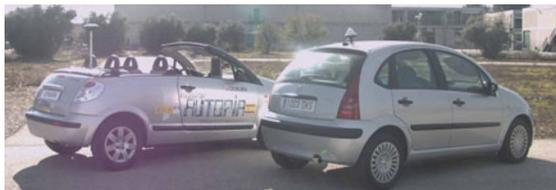
**Fig. 2.** AUTOPIA program cars. A fully-automated convertible Citroën C3 and an intelligent Citroën C3 car.
