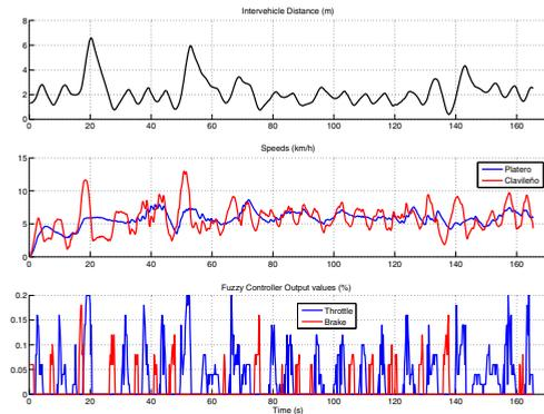
**Fig. 4.** Adaptive speed control experiment
