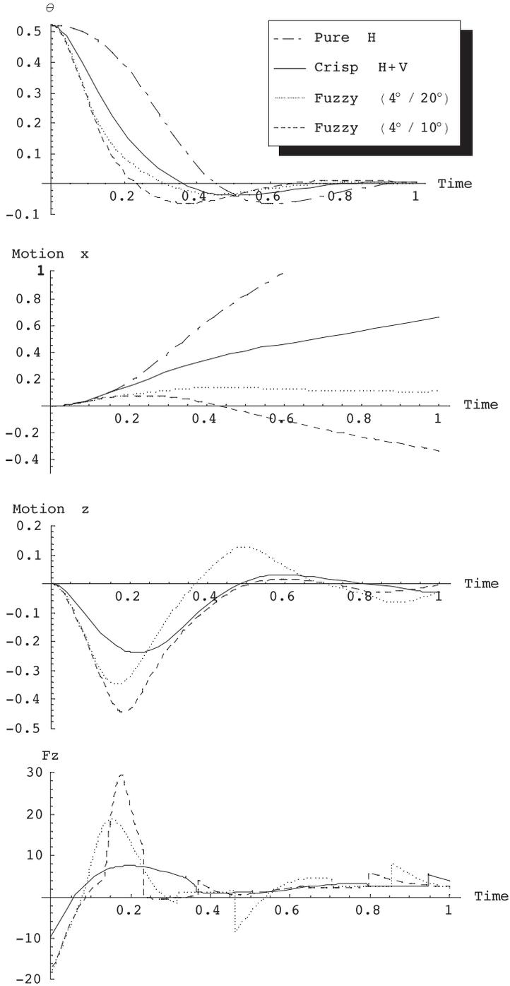
**Figure 7.** Comparative performances of pure horizontal control, crisp horizontal plus vertical control, and hybrid fuzzy control.
