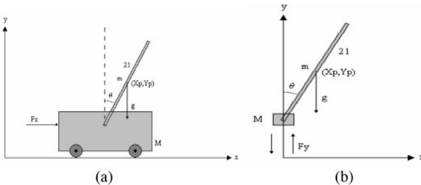
**Figure 1.** Planar inverted pendulum supported by a platform subject to (a) a horizontal force  $F_x$  and (b) a vertical force  $F_y$ .
