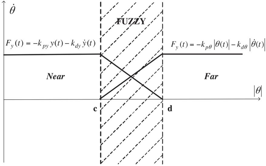
**Figure 4.** Fuzzy partition in  $(|\theta|, \dot{\theta})$  state space of the IP ( $\text{sgn}(\theta) \neq \text{sgn}(\dot{\theta})$ ).
