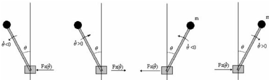
**Figure 2.** The four possible IP states. Observe the orientation of the respective feedback force.
