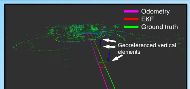
Results show how the odometry trajectory (magenta) differs from the ground truth (green), that is known thanks to a **differential GPS signal** from the car. When the car is close to the georeferenced elements (represented as RGB frames), the EKF (red) performs corrections if data association is successful. Thus, **the EKF trajectory, which coincides with odometry before noticing any known vertical element, moves towards the ground truth**.
