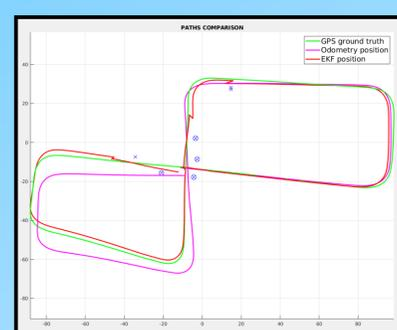
This poster presents a proof of concept for an alternative method of localization using Velodyne VLP-16, which is a critical issue in the field of autonomous vehicles. While not optimal, it has been proved to work under certain conditions, and it could be considered as a good solution in those situations when GPS signal is not accurate enough to meet the security requirements of autonomous vehicles.
