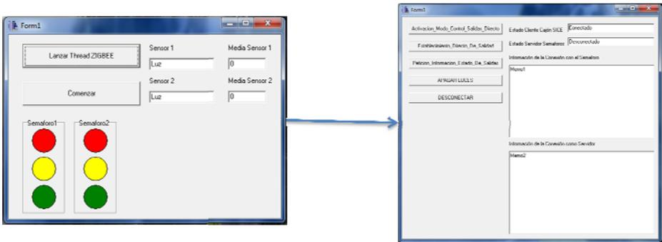
Fig. 6. The control program (left) set the traffic light to green or red depending on the vehicles detected. The traffic lights regulator is modified via an interface program (right).
