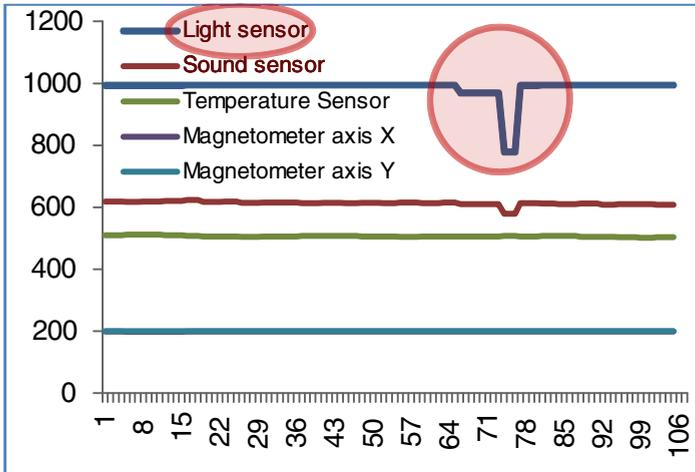
Fig. 3. Vehicle detection test: This experiment is used to choose the sensor to detect the vehicles
