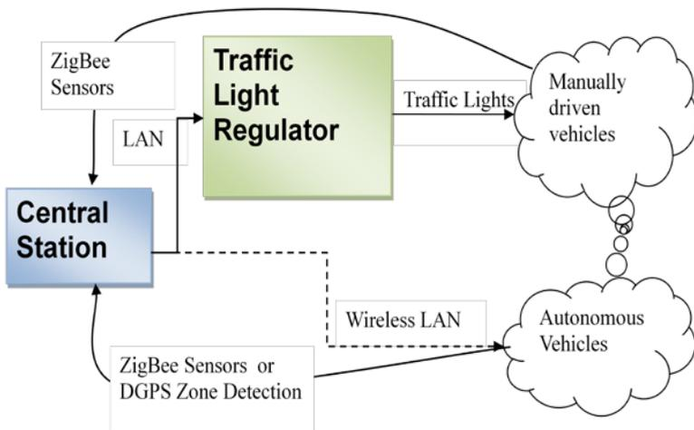
**Fig. 1.** System scheme: The central station get as inputs the positions of the manually and autonomously driven cars via the ZigBee sensors or the DGPS zone detections. And it sends as outputs orders directly to the vehicles via Wireless LAN or it modifies the traffic lights sending orders to the traffic light regulator via Local Area Network.
