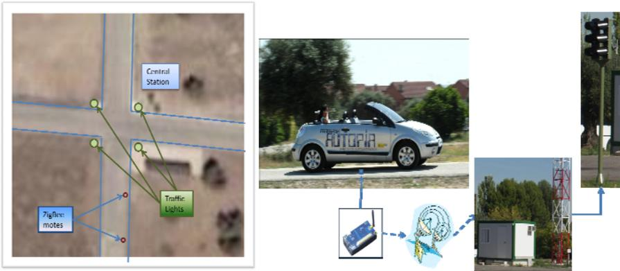
**Fig. 4.** Sensor test layout. This figure shows the placement of the ZigBee motes in the intersection (*left*) and the schema of the vehicle detection, and actuation over the traffic lights (*right*).
