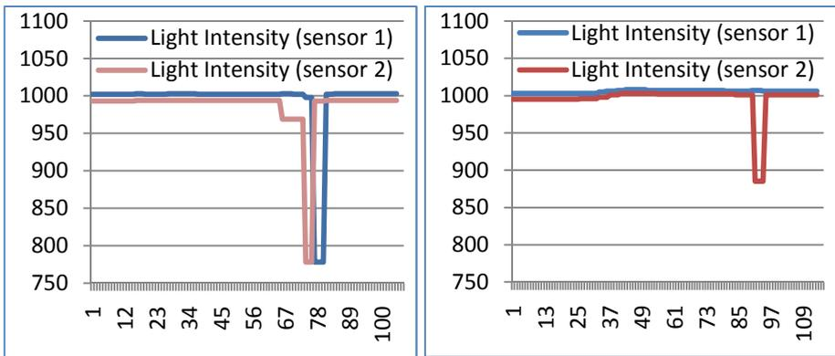
**Fig. 5.** The light intensity of both sensors decrease more than 200 cd when the vehicle goes above the sensor at 12km/h (*left figure*). When the vehicle goes at a higher speed, 35 km/h, the variation of light intensity detected is only 100 cd for the second sensor, and zero for the first sensor (*right figure*).
