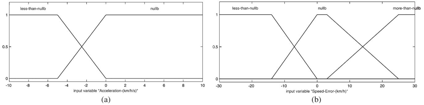
Fig. 3. Brake CC fuzzy controller input membership functions. (a) *acceleration*. (b) *speed\_error*.
