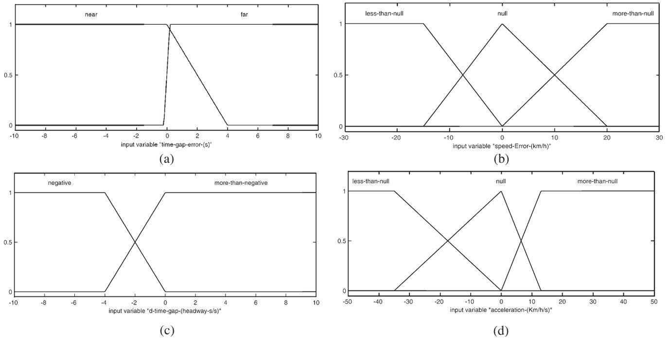
Fig. 2. ACC fuzzy controller input membership functions. (a) *time\_gap\_error*. (b) *speed\_error*. (c) *d\_time\_gap*. (d) *acceleration*.
