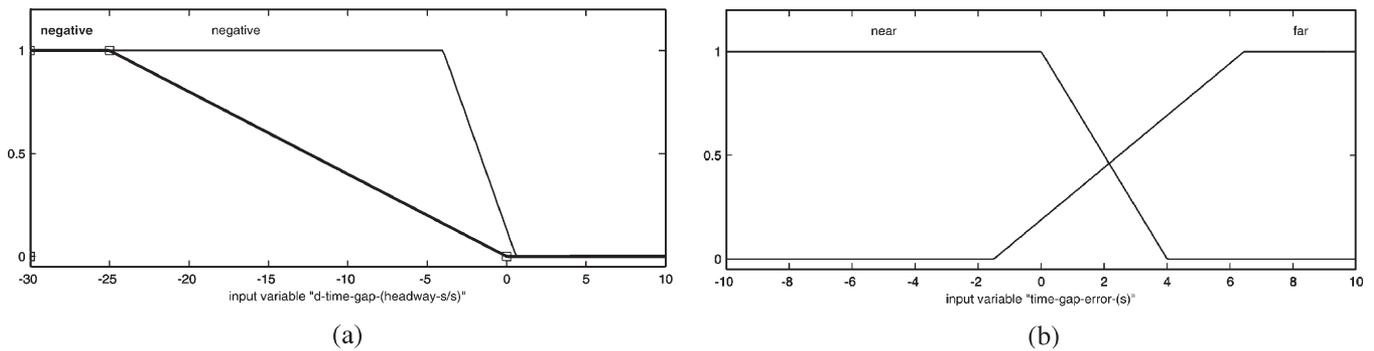
Fig. 4. ACC extended with brake pedal input membership functions. (a) *d\_time\_gap*. (b) *time\_gap\_error*.
