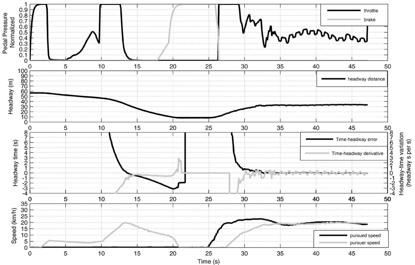
Fig. 5. ACC and Stop&Go maneuver. First experiment.
