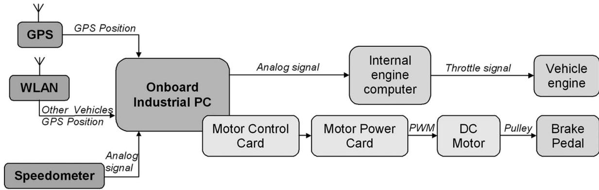
Fig. 1. Schematic description of the hardware setup.
