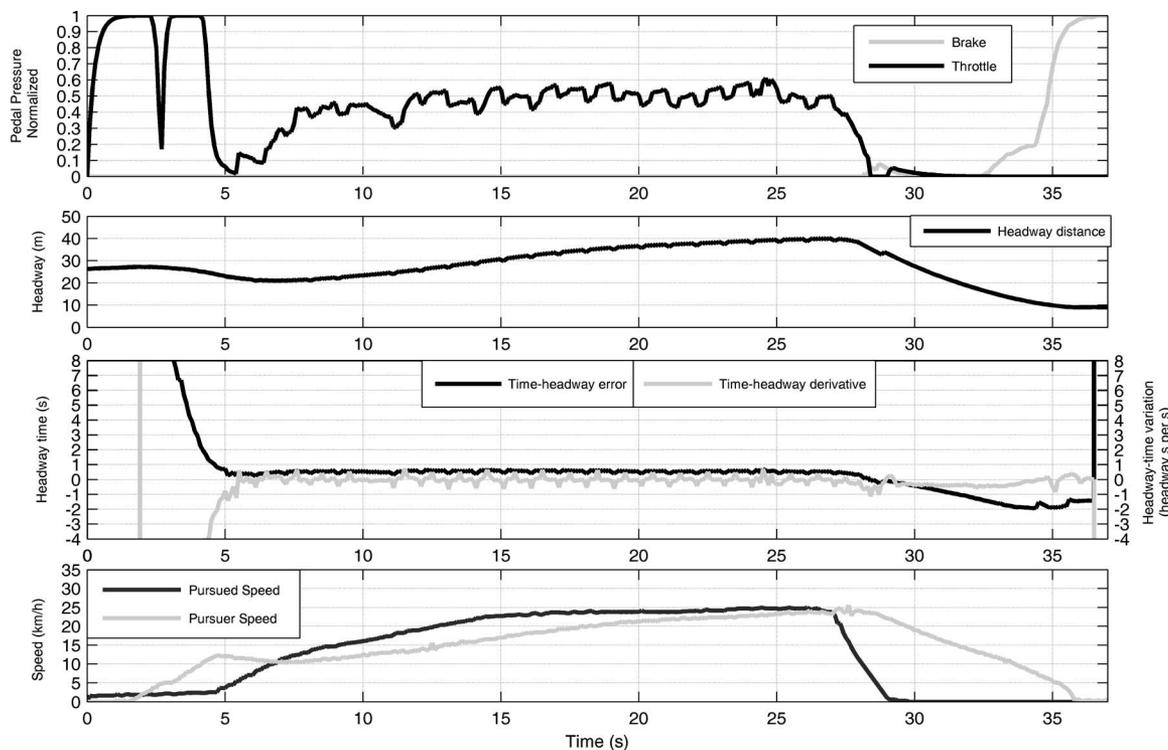
Fig. 6. Stop caused by a sudden braking action of the fore car.
