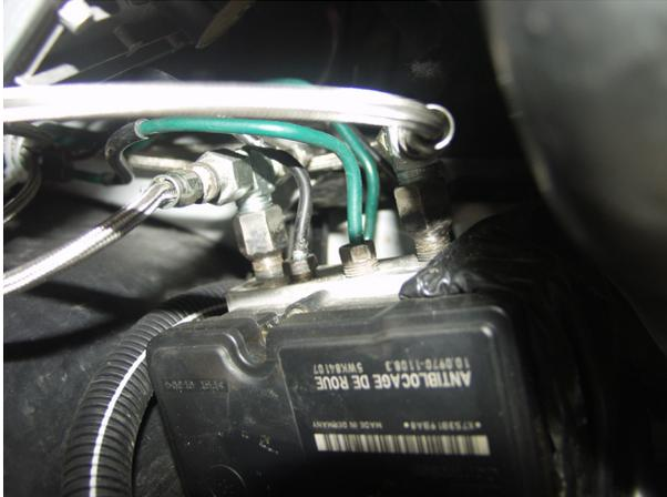
Figure 2. Locations of the shuttle valves.
