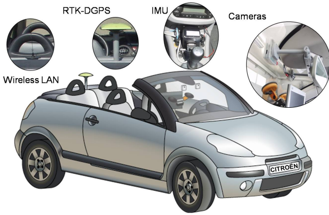
Figure 2. Citroën C3 Pluriel on-board sensors.
