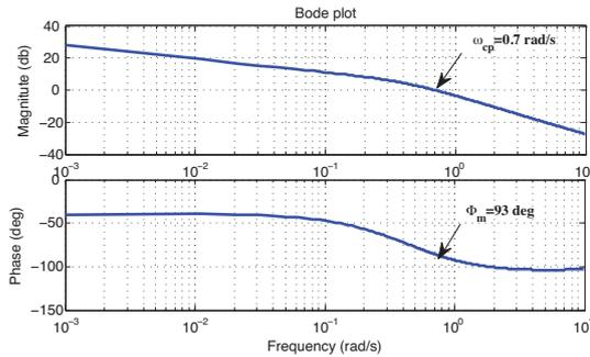
Fig. 2: Bode plot of the controlled vehicle by applying the designed  $PI^\alpha$  brake controller
