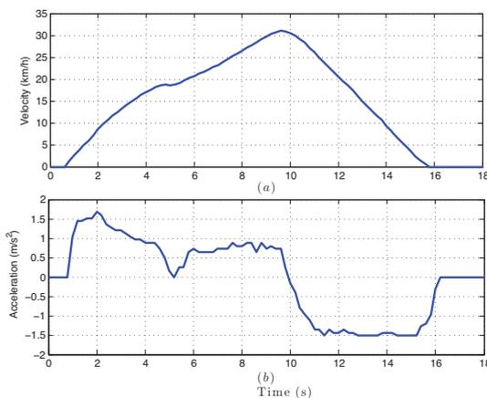
Fig. 9: Brake control results
