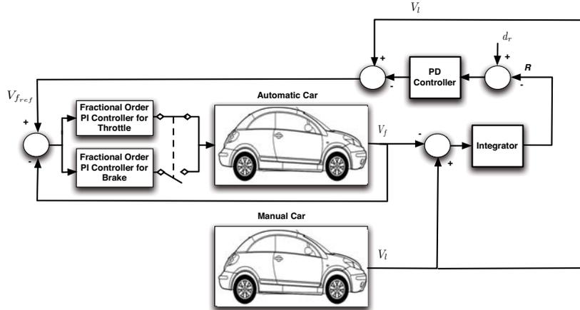
Fig. 4: Block diagram of ACC system
