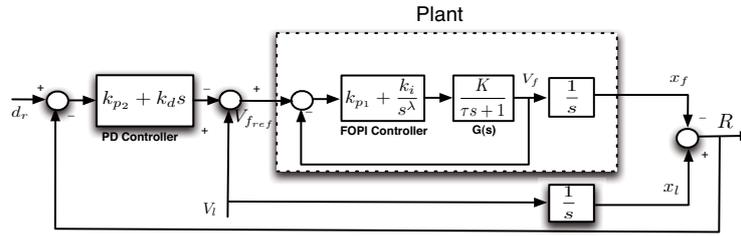
Fig. 5: Scheme of the closed loop system
